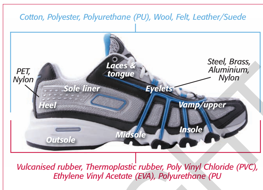
A typical sports shoe with main parts and commonly used materials.
